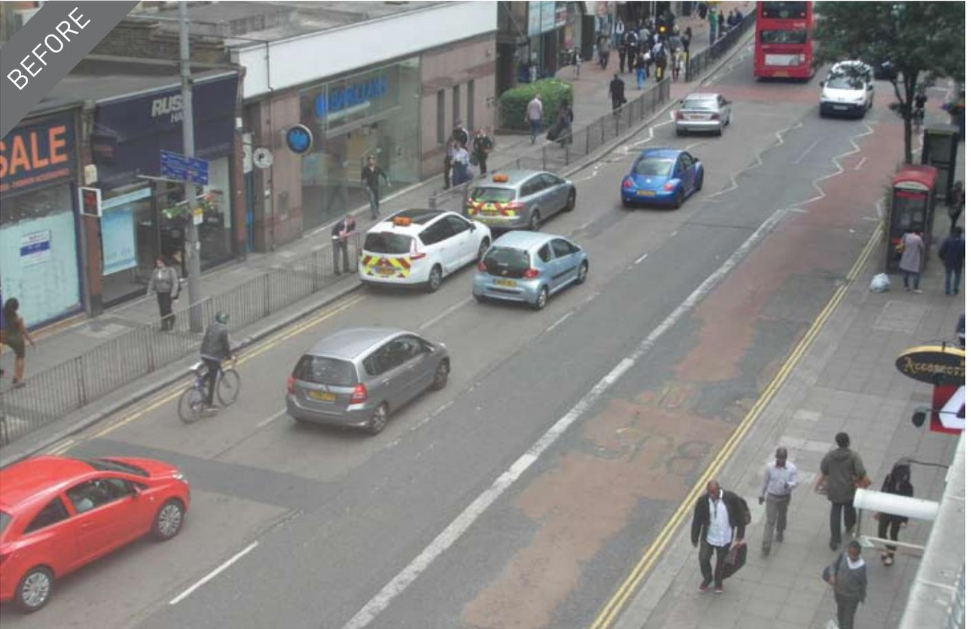
The centre of Ealing Broadway, west towards the junction with High Street: reallocating existing carriageway space - again inefficiently used at present - to create new, protected bike lanes in each direction. Removal of guard-railing will widen effective footway widths. Details of layout at eastbound bus stop will encourage cyclists to slow and create safe space for boarding and alighting passengers.
