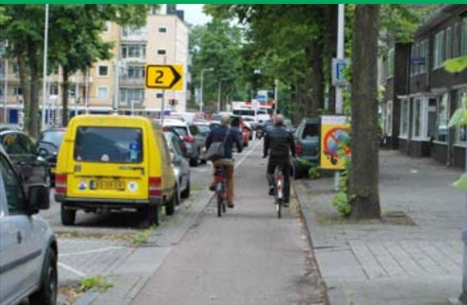
Carefully laid out cycle routes, such as this one in Utrecht, allow for on street parking but also use the parking to protect cyclists from faster moving traffic. Buffer strips also protect cyclists from car doors.
